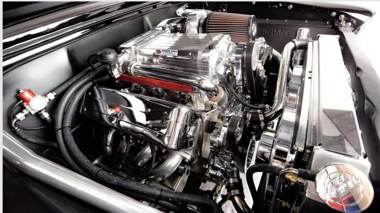
An LS2 with a Kenne Bell supercharger pumps out 700 hp. An intercooler is located below the radiator.
